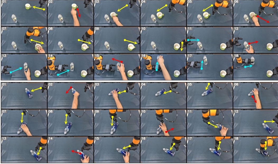
Figure 16: Qualitative examples of applying dynamic interferences during the pre-grasping execution. From top to bottom, they are segments of the dynamic closed-loop grasping phase of tasks pouring and reorient+unscrew, where each object is manually disturbed from one to three times. The red arrow indicates the direction of the manually moved object (interfering). The cyan arrow and yellow arrow indicate the movement direction of the left and right robotic arms (chasing) respectively. Best to view after zooming in.
