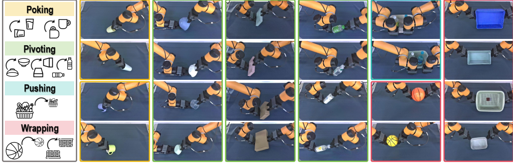
Figure 3: Examples of four non-prehensile skills instantiated with different tasks and diverse objects.
