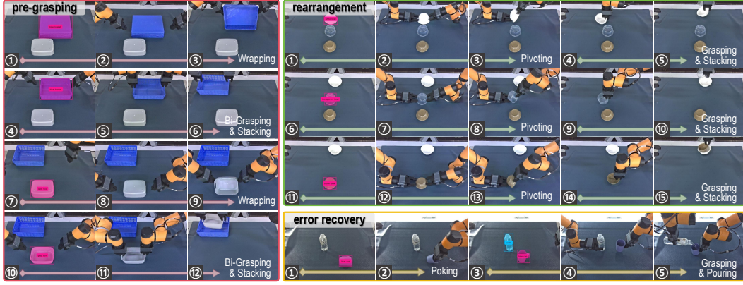
Figure 4: Examples of utilizing learned non-prehensile skills to boost complex manipulation tasks.
