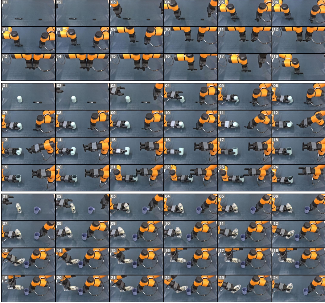
Figure 10: Examples of synchronized dual-arm movement. Segments from top to bottom are tasks plugging, inserting, and pouring, which have relatively high dual-arm synchronizability.
