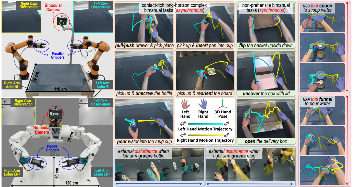
Fig. 1. Our proposed YOTO++ (You Only Teach Once) enables cross-embodiment deployment (from the contralateral to humanoid dual-arm setups), and facilitates diverse bimanual tasks including asynchronous, synchronous and tool-using scenarios, with closed-loop control under external disturbances during pre-grasping. Notably, it needs only the one-shot observation of a third-person binocular camera to extract the fine-grained motion trajectory of human hands, which can then be utilized for the dual-arm coordinated action injection and rapid proliferation of training demonstrations.
