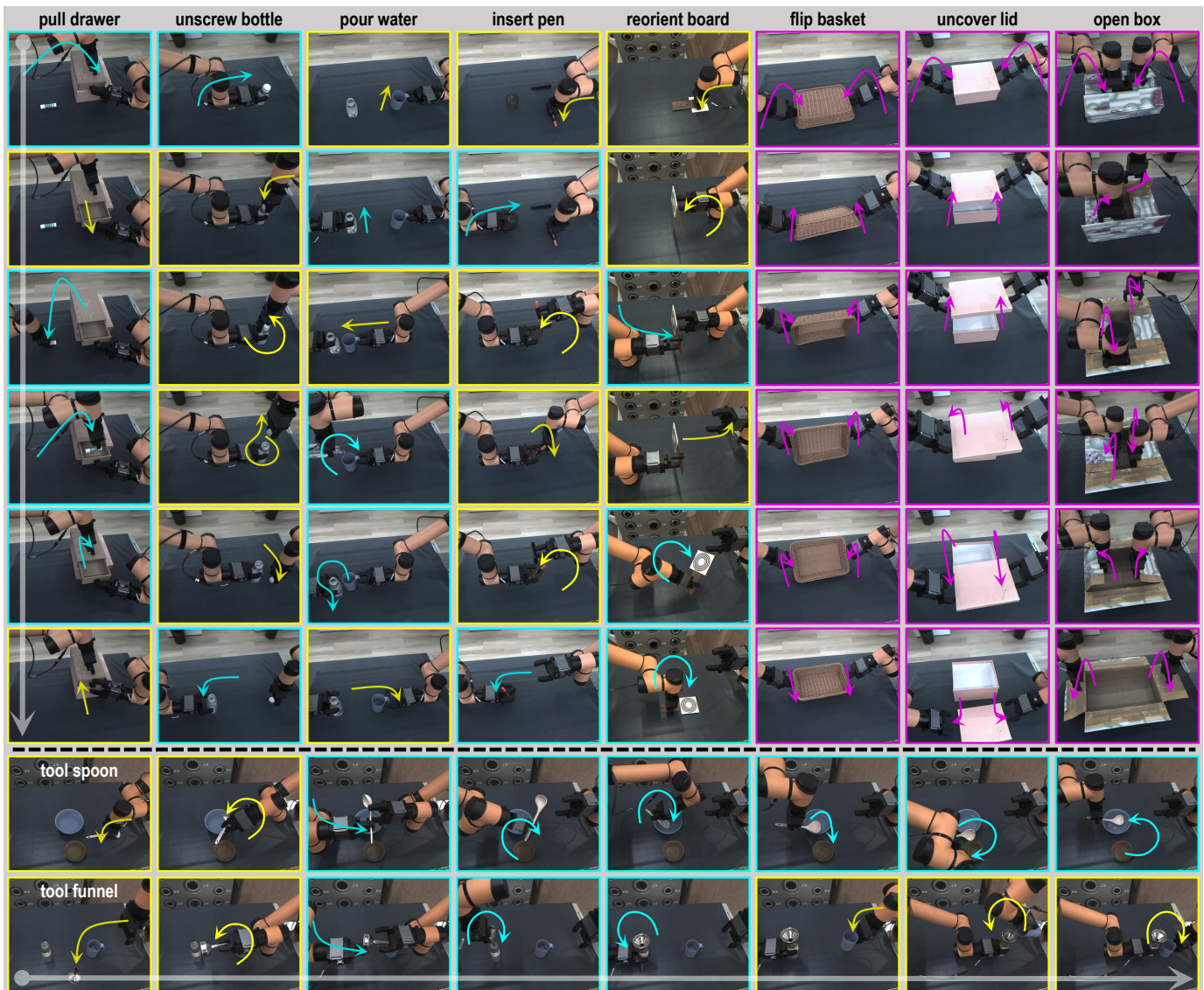
Fig. 9. Visualization of ten bimanual tasks performed on real robots. We use different colors such as teal, olive and purple to distinguish frames of left arm, right arm and both arms, respectively. Arrows are artificially added to show movement trends. It is best to zoom in to view the details.
